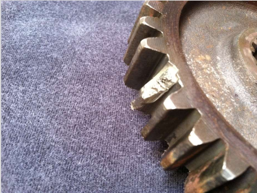
Gear failure from fatigue
